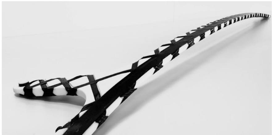
FIGURE 1 Prototype of the roof frame, implemented using AdditiveCarbon (© Cikoni)
