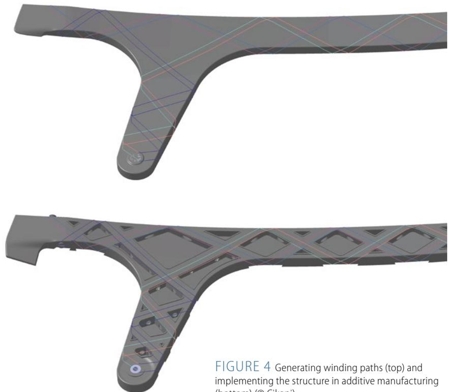
FIGURE 4 Generating winding paths (top) and implementing the structure in additive manufacturing (bottom) (© Cikoni)
