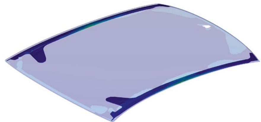
FIGURE 3 FEM model of the reference assembly as the starting point for component sizing (© Audi)
